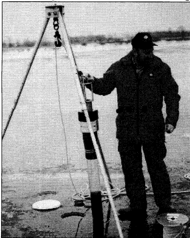
Collecting sediment samples through the ice
